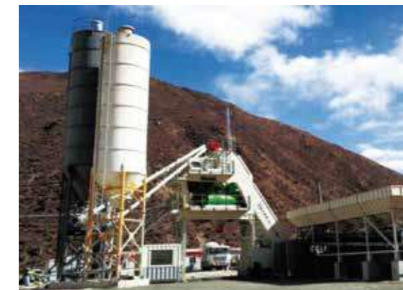
西宁高速HZS120VG(工程提斗站) HZS120VG (engineering buck-type mixing plant) for Xining expressway
