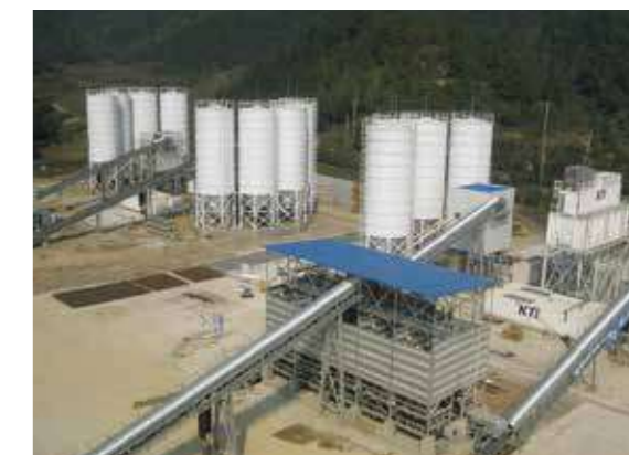
陆丰核电4HZS150VG(核电站) 4HZS150VG (mixing plant for nuclear power plant construction) in Lufeng nuclear power plant
