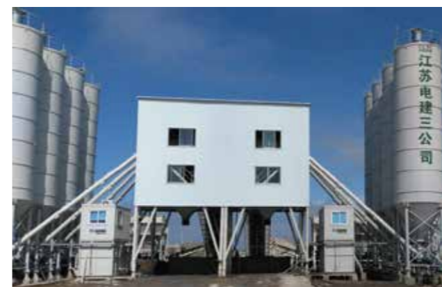
江苏电建2HZS180V (快搬站) 2HZS180V (quick-handling mixing plant) in Jiangsu Electric Power Construction Co.,Ltd.
