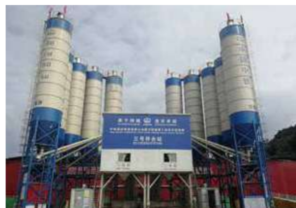
中老铁路样板工程2HZS120V(高铁工程站) 2HZS120V,(engineering plant for high-speed railway ) Sample Railway in Laos,China
