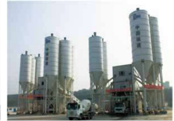
南京中核2HZS180V (标准商混站) 2HZS180V (standard concrete plant) in Nuclear Group, Nanjing
